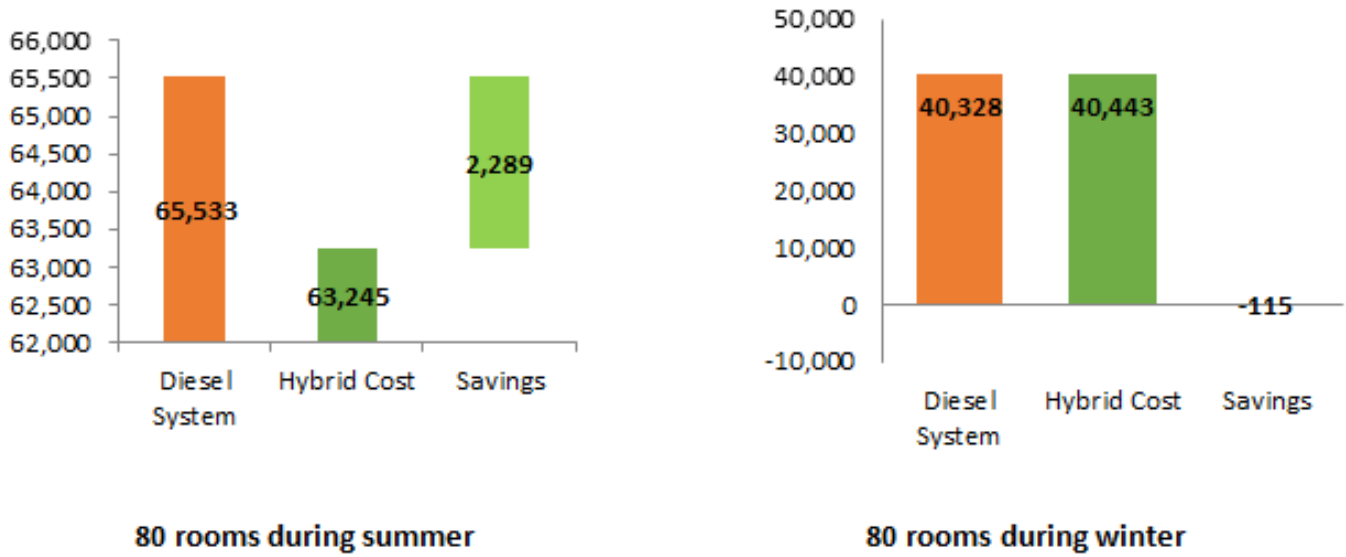
Fig. 21: Scenario 2 — 80 rooms during summer and winter, using an average rate of 2.74 kWh/liter
